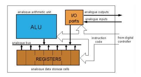
From this image of architecture of microprocessor it can be easily seen that it have registers and ALU as processing unit and it does not have RAM, ROM in it.
